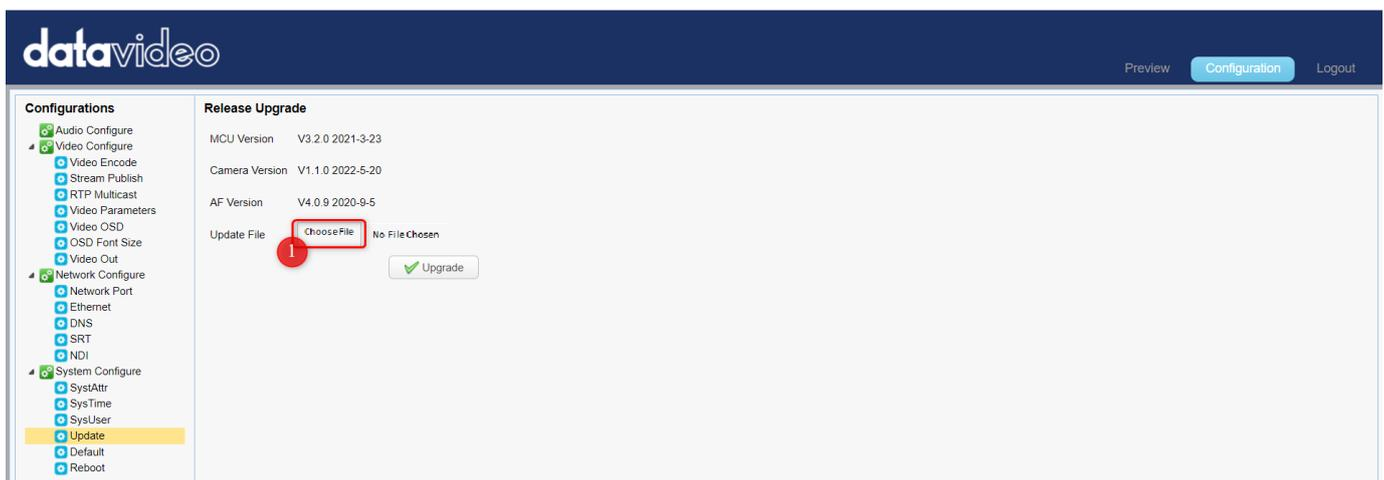
2. After the latest MCU firmware is selected, please press the “Open” button, and then you can see that the latest MCU firmware “D-PTC-140\_NDI\_ARM\_V3.2.2\_20220422.mrg” is selected.
