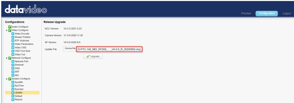
3. After the latest camera & AF firmware is selected, please press the “Upgrade” button. After that, the firmware update procedure will be started automatically.
